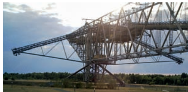
F60 – mobile overburden conveyor bridge located in the Lower Lusatia
